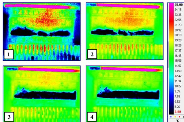
**Figure 3.** Thermographs of a specimen. We can notice the Transition from the Unstable Heat Flux Phase (1-3) to Stable Heat Flux Phase (4)
