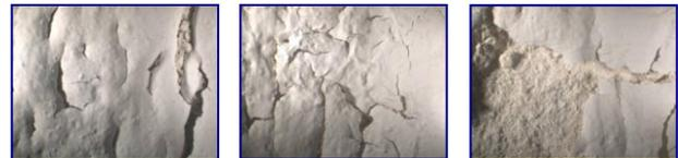
Figure 2. Etics Specimens with Cement Coating Failure
