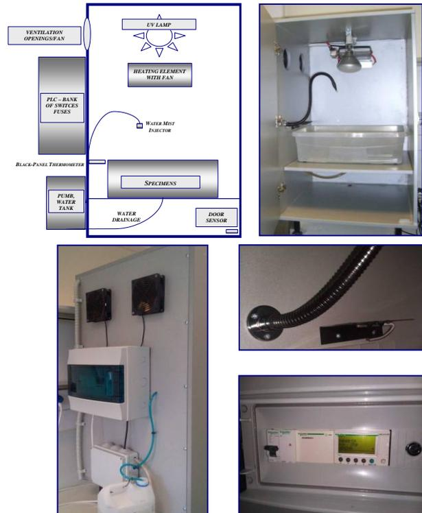
Figure 1. – Constructed Chamber/Apparatus for UV Stress Test
