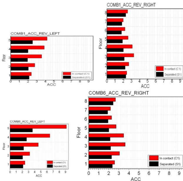
Figure 5. Max. floor accelerations: BC#1 - BC#6 and REV earthquakes.
