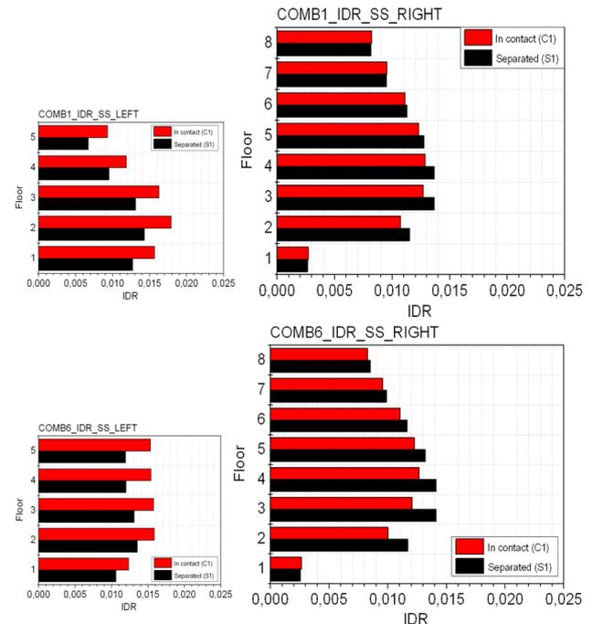
Figure 8. Max. interstorey drifts: BC#1 - BC#6 and S-S earthquakes.
