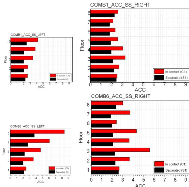
Figure 6. Max. floor accelerations: BC#1 - BC#6 and S-S earthquakes.
