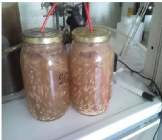
**Figure 1.** Reactors supplied with PVA beads
