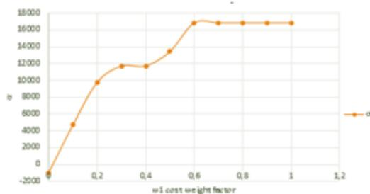
As observed, the smallest energy differences are in the area  $w1 = 0,2$  to  $0,4$ . This means that our empirical selection achieves the smaller energy differences than the respective best solutions for  $w1 = 0,2$ ,  $0,3$  and  $w1 = 0,4$ , i.e emphasizing respectively 80%, 70% and 60% savings energy.
